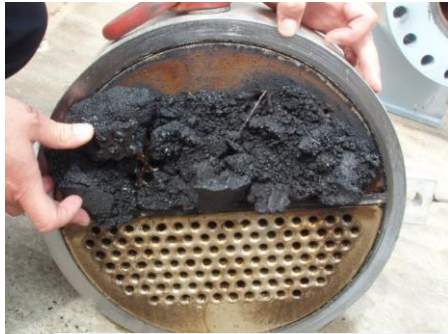
Using Mineral Oil-based Lubricants Results in Deposit Formation
